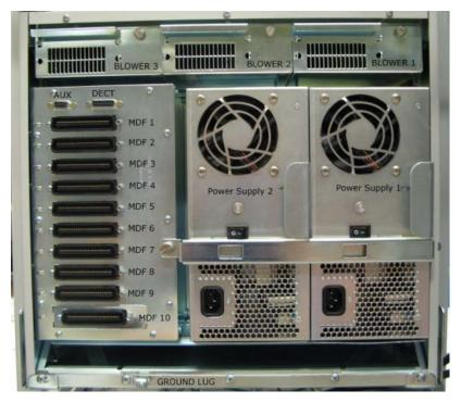
Figure 9: MG 1010 rear components
