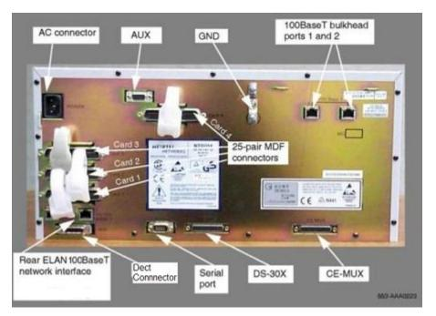
Figure 4: Rear components in the Media Gateway 1000E
