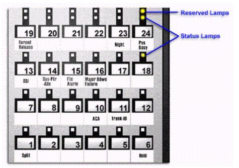
Figure 9: Console feature button layout
