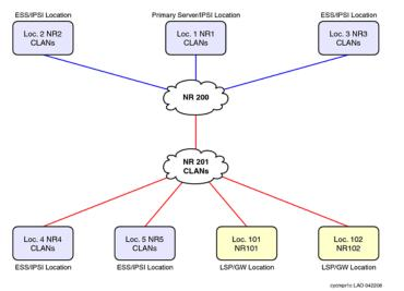
Figure 3: Improved configuration for unwanted C-LANs using the enhanced AGL feature
