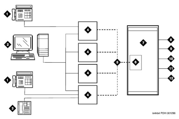
Figure 12: ISDN—BRI Personal Computer interface configuration (Group 2)
